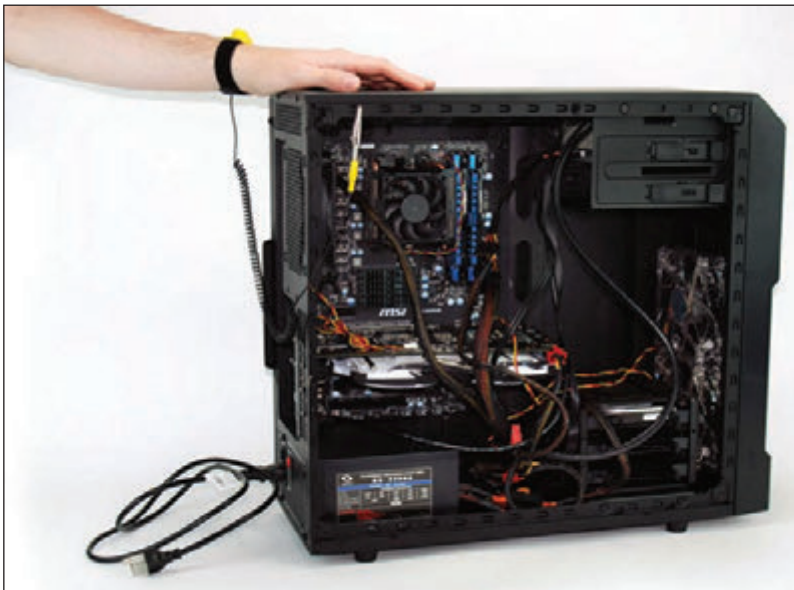
Figure 1-2 An ESD strap, which protects computer components from ESD, can clip to the side of the computer case and eliminate ESD between you and the case
