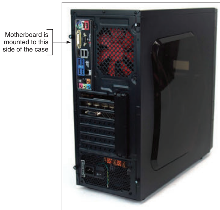
Figure 1-7 Decide which side panel to remove
