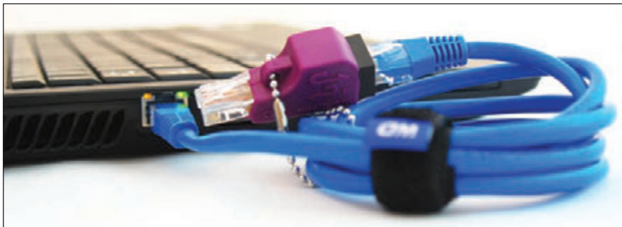
Figure 1-5 A loopback plug testing a network port and network cable
